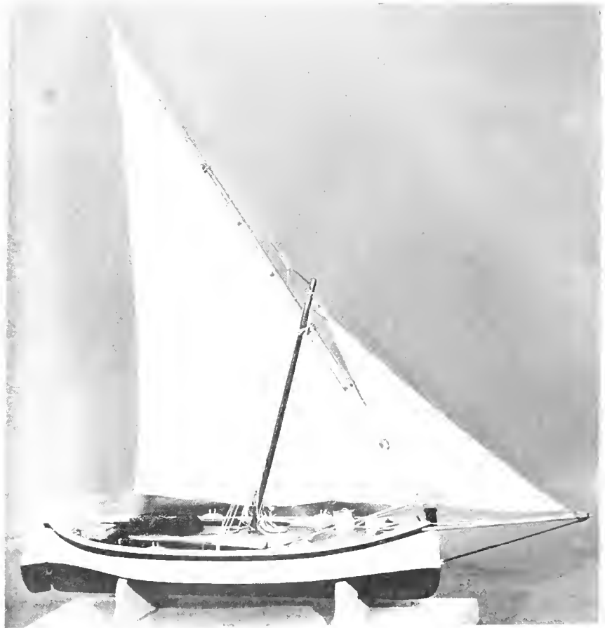
SAN FRANCISCO FISHING BOAT of 1876, developed by local fishermen of Italian descent. Rigged model USNM 22214. (Smithsonian photo 45606-b.)
